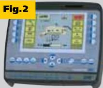
The monitor is connected to the spreader control panel, after which it starts regulating the fertiliser dosage in accordance with the GPS position. The spreader automatically regulates the dosage of fertiliser introduced. Ammonium phosphate and potassium fertilisers are introduced alternately.
