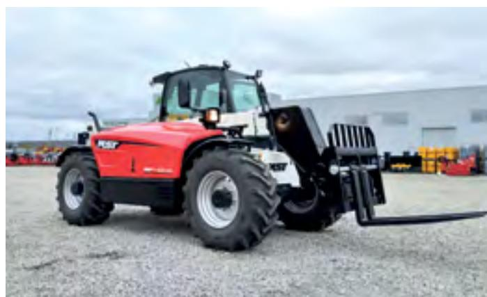
an articulated frame, with a rated lifting capacity of 3 t and an operating weight of up to 10,250 kg. Besides the three packages available for the machine, it can be custom-tailored to suit farm's individual needs. The model has already proven
