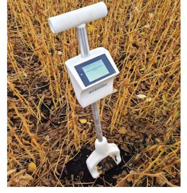
'The system has a built-in GPS-module to determine the precise coordinates of the explored area, which is key to establishing the differences in the nutrient content across the field. Besides, the lab features embedded field mapping software which provides fertiliser application guidelines. All the data is immediately uploaded to the server and promptly processed. The user has an instant access to the records via a dedicated app', continues Artyom Novikov.
