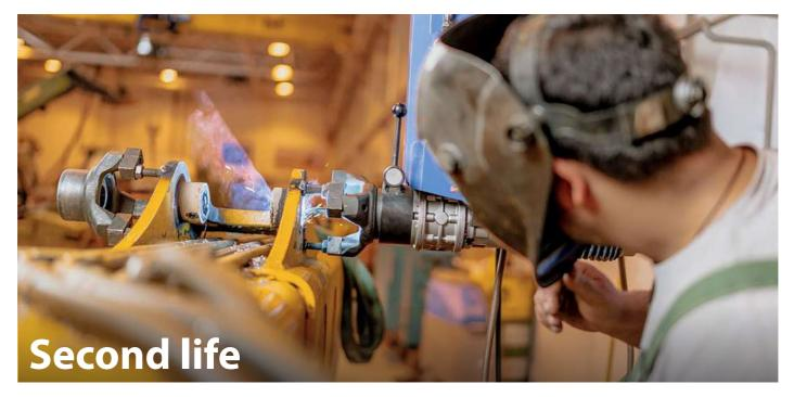
The specialists of EkoNiva machinery dealing holding give equipment a second life. Within a few hours, service technicians can restore worn-out holes and articulated joints in farm machines using methods of metal overlay welding and boring.
