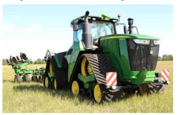
wider than on rival machines, the wrap angle, which is 24 degrees larger, and the 60% higher belt tension prevent slippage.'
