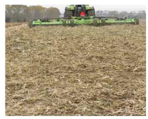
Corn stalk mulching with the Schulte rotary mower is carried out immediately after the combine harvester has passed
