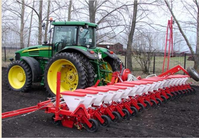
The design of this drill uses modular concept. This makes changing of sowing units, coulters and press wheels easy. The wheels of this planter are located in front of sowing units allowing to change a row width easily from 30 cm up to 80 cm. The sowing units are driven from a central drive system working via the idler wheels. The drive unit is mounted externally on the side of the
