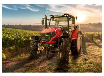
features a 116 hp 4-cylinder diesel engine with Turbo/ Intercooler from Deutz and the Common Rail fuel injection system. The unit is enhanced with the 4-speed synchronised PowerShift transmission produced by ZF with 32 forward and 32 reverse gears, electro-hydraulic gear shifting and a four-wheel drive.
