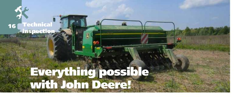
Danilovka Farm LLC is an advanced seed production enterprise in the Kaluga oblast which is constantly introducing modern technologies and carrying out experiments. This year was no exception. For the first time the farm used the No-Till technology, employing the John Deere 1590 drill.
